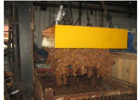
Loose Parts Lifting
